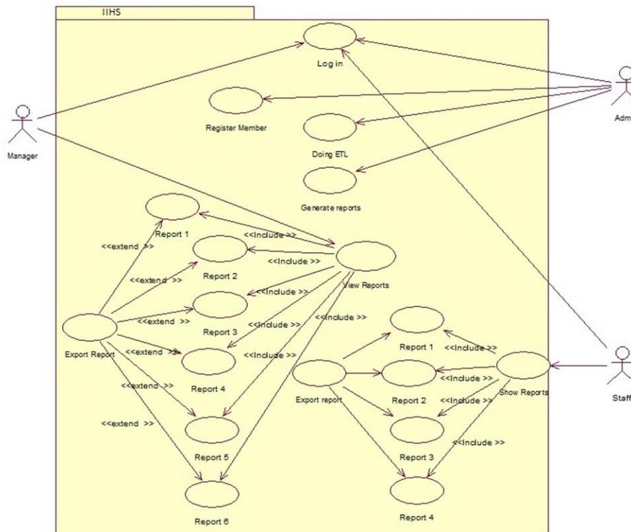
Figure 1. Use Case Diagram Level 1 for IIHS
