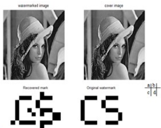
Figure 3: Image to demonstrate watermarking process. (a) The watermarked image. (b) The host image. (c) The recovered watermark message. (d) The original watermark.
