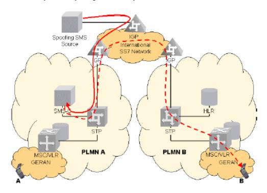
Example: SMS Spoofing in a Cellular provider's Infrastructure
