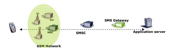
Figure 1: A diagrammatic representation of the SMS Network components
