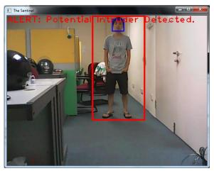
Figure 6. Detection of a Potential Intruder
