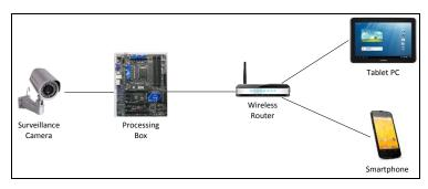
Figure 3. Systems Architecture of The Sentinel
