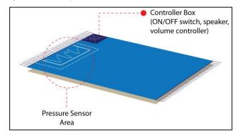
Figure 1. Smart Prayer Mat Equipped with Pressure Sensor
