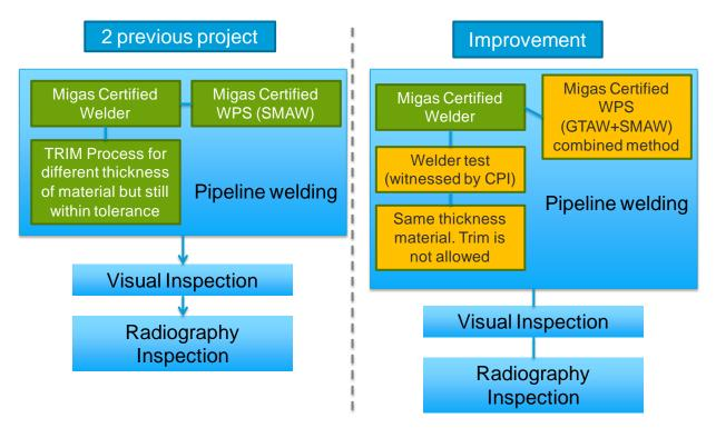
On the two previous works, the contractor employed welders with qualification that proven by welder certificate. In the new process, those welders are test again and witnessed by the Company representative to ensure the welder performance. In the welder test, some welders failed and the consequences is grounded, not allowed to weld the line pipe. Along grounded time, the welding is coaching by the company representative in weekly, and after they confidence can propose another welder test.
