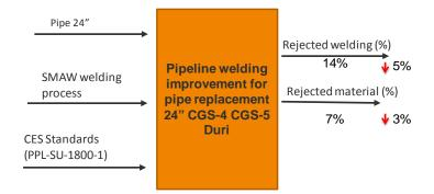
IPO Diagram constructed as above for this improvement process. The input is material line pipe 24 inch, the welding process, and the standard related with welding process. The expected output is rejected welding decrease from 14% to 5%, and rejected material decrease from 7% to 3%.
