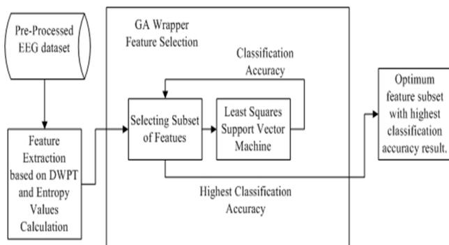
Figure 1 The proposed EEG emotion recognition model
