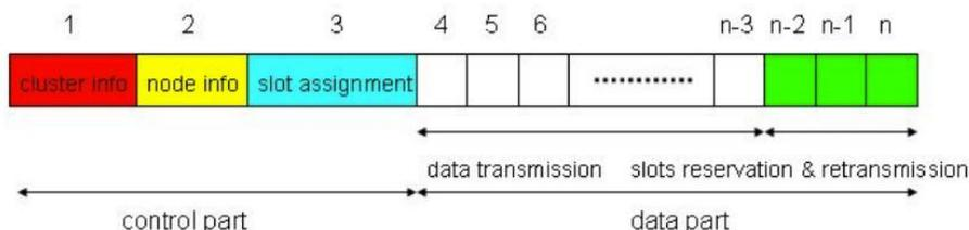
Figure 5: M-TDMA working principle [36]
