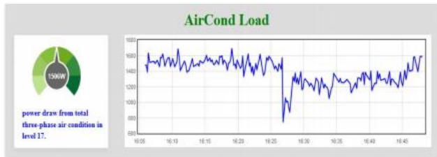
Figure 14: Air conditional power consumption
