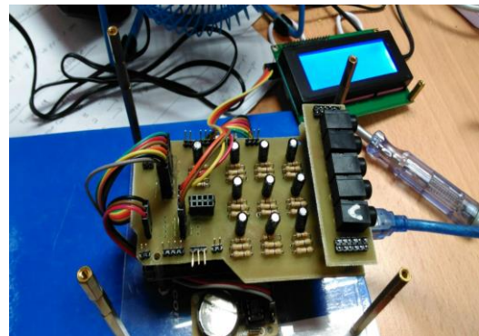
Figure 6: Complete energy monitoring device
