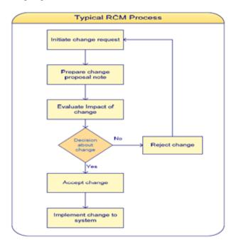
Figure 1: Typical RCM process flow [7]
