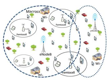
Figure 2: Heterogeneous Multi-RAT Environment
