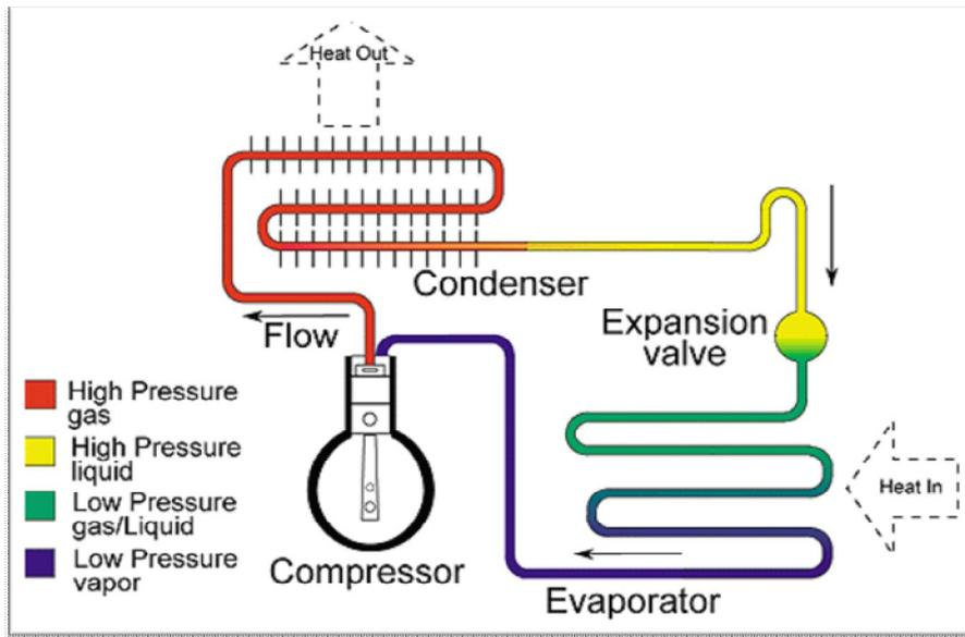
Figure 1- Basic Operation of Air Conditioning Units [23]
