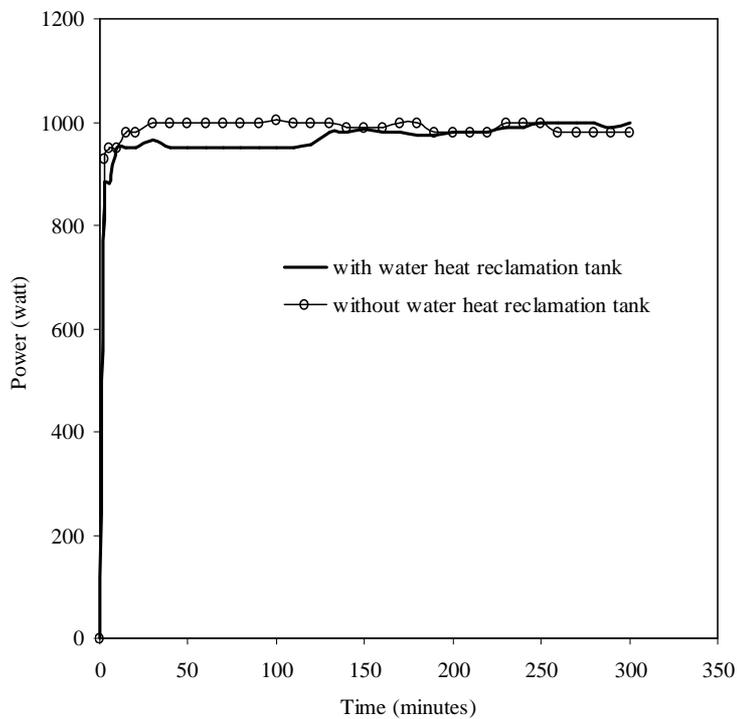
Figure 4- Power Consumption of the Waste Heat Scavenging System
