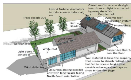
Figure 1: The design for an energy efficient green house
