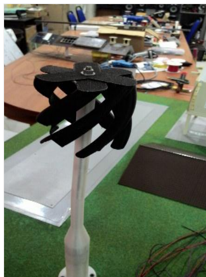
Figure 5: Vertical axis wind turbine custom made using 3D printer
