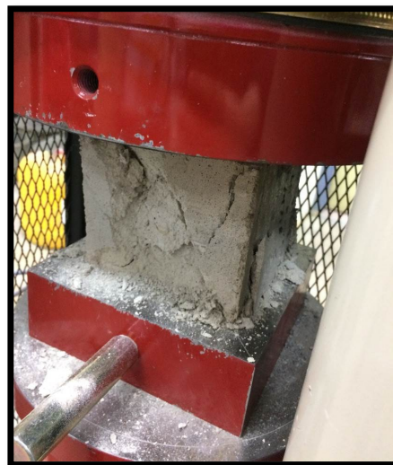
Fig. 2. Compression test setup in accordance with BS12390
