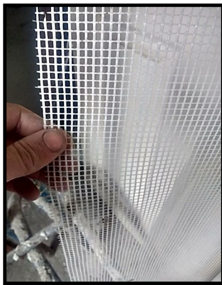
Fig. 1. Interlaced fiberglass mech of 160gsm
