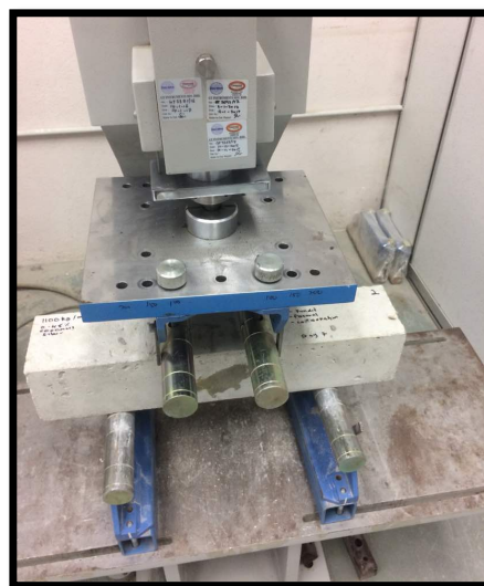
Fig. 3. Bending test setup corresponding to BS1521
