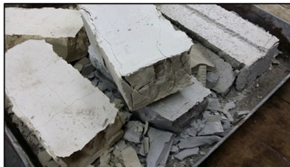
Figure 2: Condition of Bricks Sample after Compressive Test
