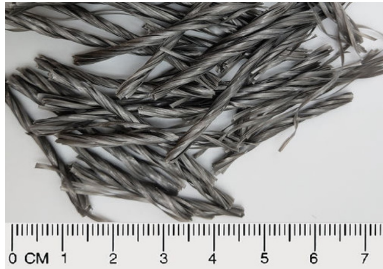
Figure 1. Polypropylene twisted bundle fiber (PTBF) of 37 mm in length.
